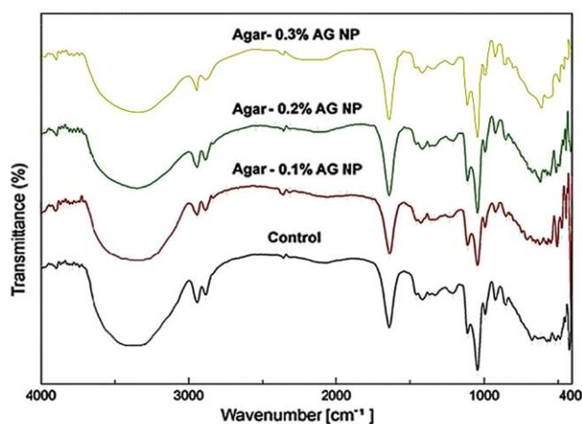
**Figure 3.** Fourier transform infrared spectroscopic analysis of control, Agar - 0.1% AG NP, and Agar - 0.2% AG NP films. Control: film formulation without AG NP; Agar - 0.1% AG NP: 0.1% AG NP/100 mL film formulation; Agar - 0.2% AG NP: 0.2% AG NP/100 mL film formulation; Agar - 0.3% AG NP: 0.3% AG NP/100 mL film formulation; and  $\text{cm}^{-1}$ : centimetre inverse.
