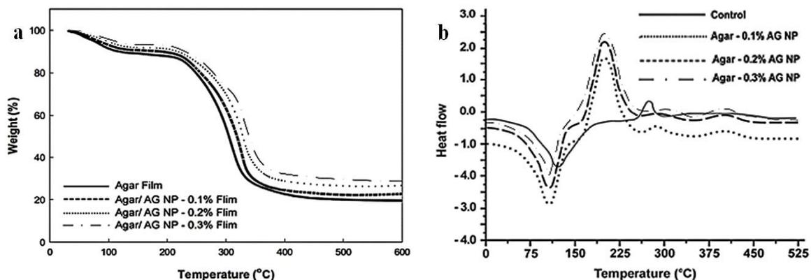
**Figure 4.** (a) Thermal stability testing of control and developed test films. (b) Differential scanning calorimetry of control and developed test films. Control: film formulation without AG NP; Agar - 0.1% AG NP: 0.1% AG NP/100 mL film formulation; Agar - 0.2% AG NP: 0.2% AG NP/100 mL film formulation; Agar - 0.3% AG NP: 0.3% AG NP/100 mL film formulation; and °C: degree Celsius.
