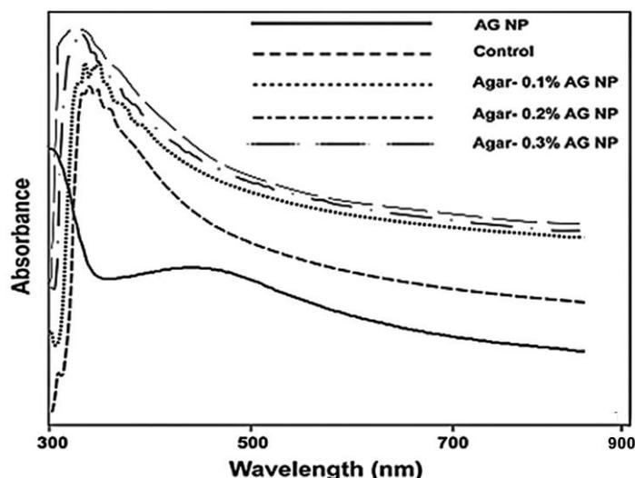
**Figure 2.** UV-Vis spectrum of synthesised AG NP from *Gracilaria canaliculata*, control film formulation, and test film formulations. Control: film formulation without AG NP; Agar - 0.1% AG NP: 0.1% AG NP/100 mL film formulation; Agar - 0.2% AG NP: 0.2% AG NP/100 mL film formulation; Agar - 0.3% AG NP: 0.3% AG NP/100 mL film formulation; and nm: nanometre.
