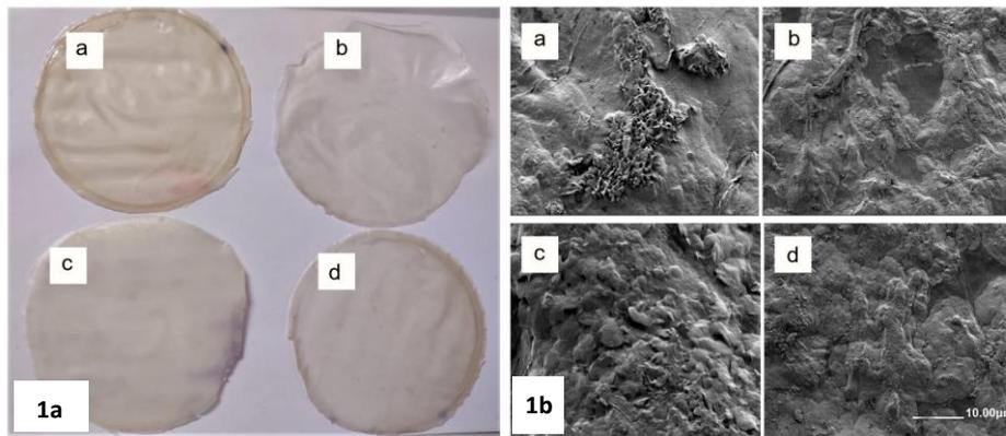
**Figure 1.** (1a) Image of control and developed test films. (1b) SEM images of control and developed test films. (a) Control: film formulation without AG NP; (b) Agar - 0.1% AG NP: 0.1% AG NP/100 mL film formulation; (c) Agar - 0.2% AG NP: 0.2% AG NP/100 mL film formulation; and (d) Agar - 0.3% AG NP: 0.3% AG NP/100 mL film formulation.
